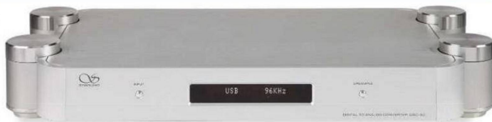
ABOVE: The display indicates the upsample mode rather than incoming rate while the rotary volume control (front right pillar top) acts on the headphone output, not the line outputs
